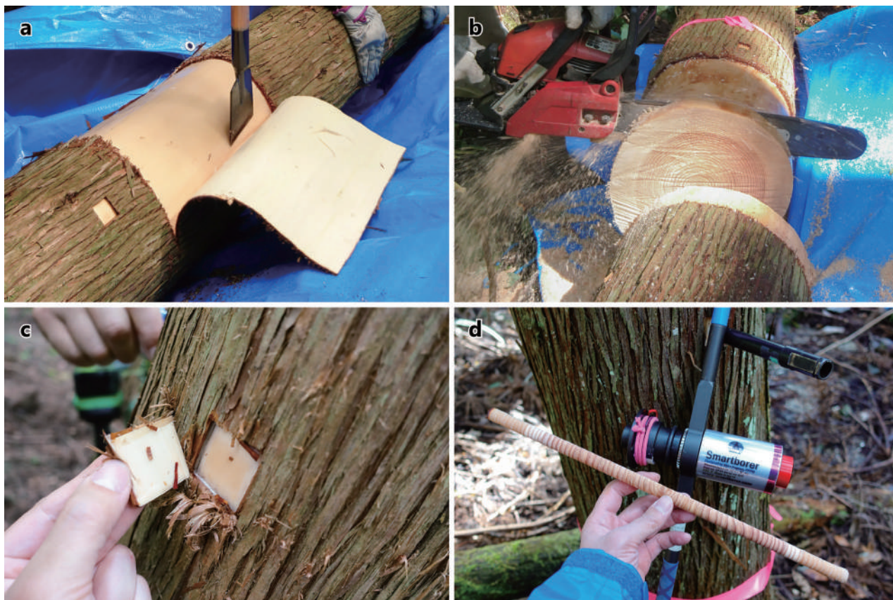
Photo 1. Sampling of (a) bark from the entire circumference of a tree stem, (b) a wood disk, (c) a bark piece, and (d) a wood core.
